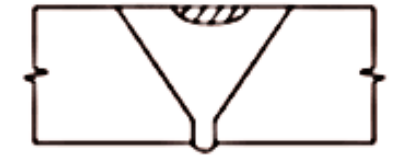
17 Transverse Crack In Single Vee, flush crown MT/PT, UT
