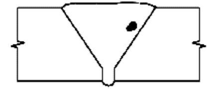
37 Slag Inclusion In Single Vee (weld groove area) UT, RT
