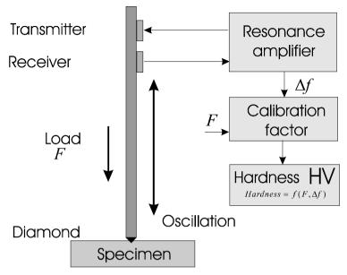
The advantages of the UCI method are the ease of automation and the very good reproducibility of the hardness readings. The reproducibility of the measurements is better than with optical methods of hardness testing because the total area of contact (proportional to d²) enters into the measurement and not only the diagonal d or a diameter. Moreover the measurement results are independent from the subjective view of a single examiner and the test is very fast executable.
