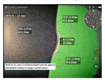
The next example shows a tip blend. A radius gauge circle is positioned over the "blend-out" position. It is sized to conform to a known acceptance radii for the well-known aero engine type. This bisects the blended material and therefore indicates that further material needs to be removed.
