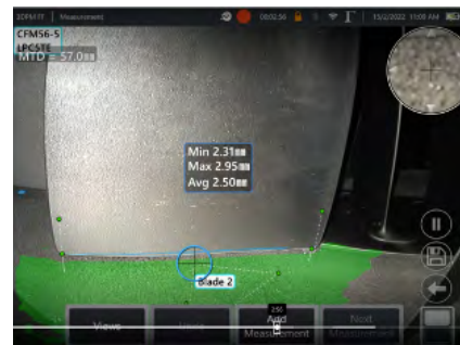
Image 3: Blade tip clearance measurement used with Blade Counter.
